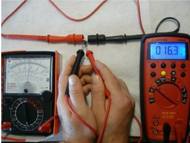
**With analogue meters black test lead on the anode pin and the red test lead on the cathode pin the DMM now shows a low resistance of 16.3 ohms between the collector and emitter.**
